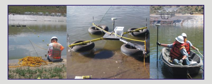
Leak detection in GeoMembrane type products is a highly effective and cost competitive method to assess HDPE and PVC liner integrity and can locate very small tears in these liners are used in a variety of industries such as solid waste (landfills), water containment facilities, mine heap leach stacks, and leachate ponds.
