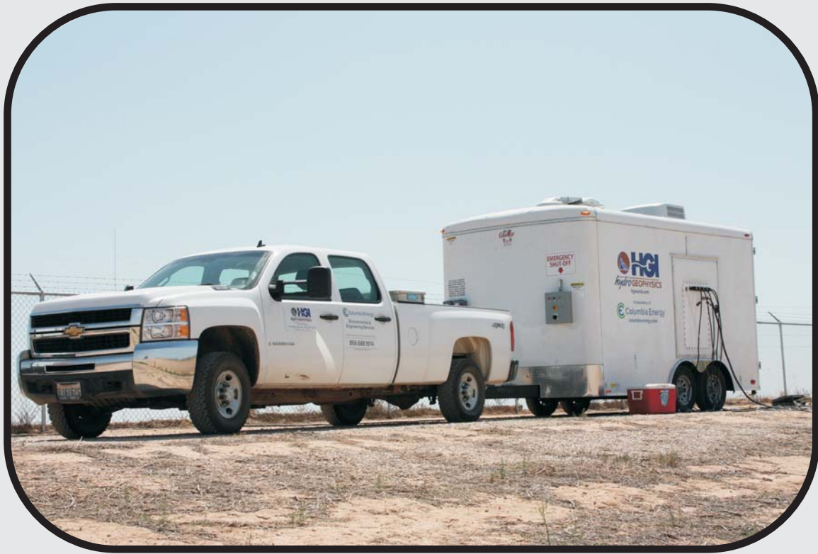
Geotection - Trailer Mounted Resistivity Acquisition System
