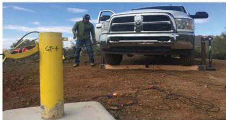
Downhole shear-wave survey for V s30 measurement
